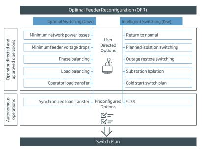
to continuously perform a load flow analysis for each time slice to detect the occurrence of violations. Violations found are presented to the operator in a schedule showing the details for the feeder.
